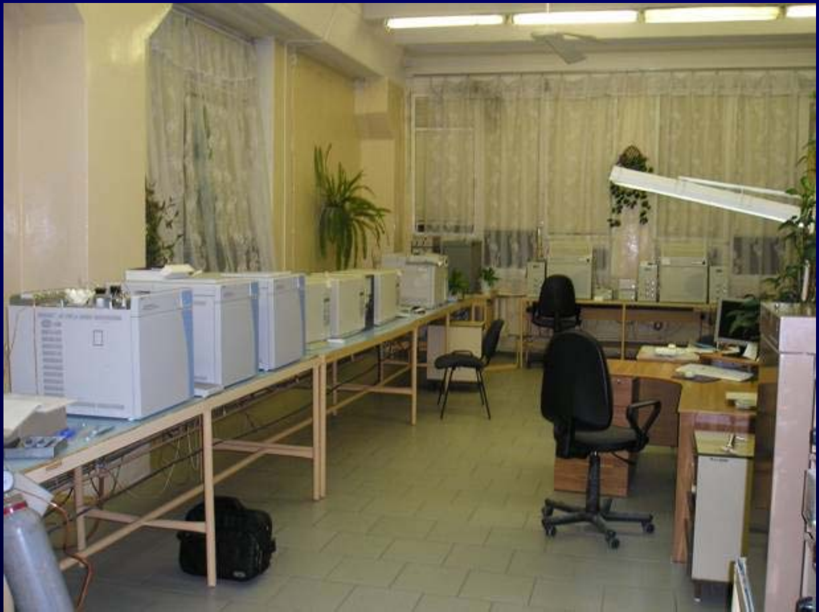
Control laboratory in JS «Nevynnomusky Azot» (Russian Federation) . UniChrom from one PC controls simultaneous: Crystal-5000 ( 3 ), Crystall-2000M ( 3 ), HP6890N ( 1 ), Tswett-800 ( 2 ), Tswett-100 ( 3 ).
